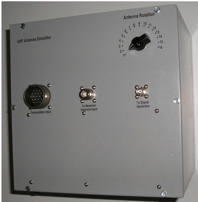
The 400041-20 radio direction finding antenna simulator was designed primarily for testing DF receivers. It operates between 100 and 200 MHz.
