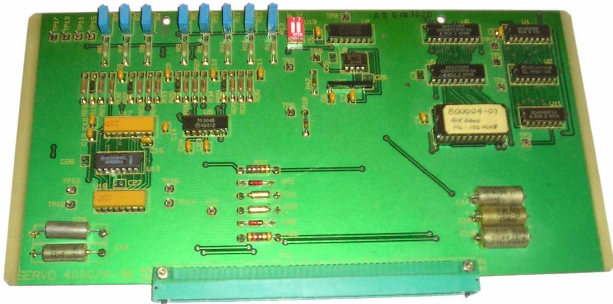
Fig.1 A5 Tuning Control Assembly 400074-36
