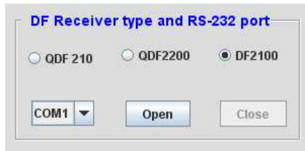
Fig.5 DFRS-2100 Selecting DF receiver type and COM port
