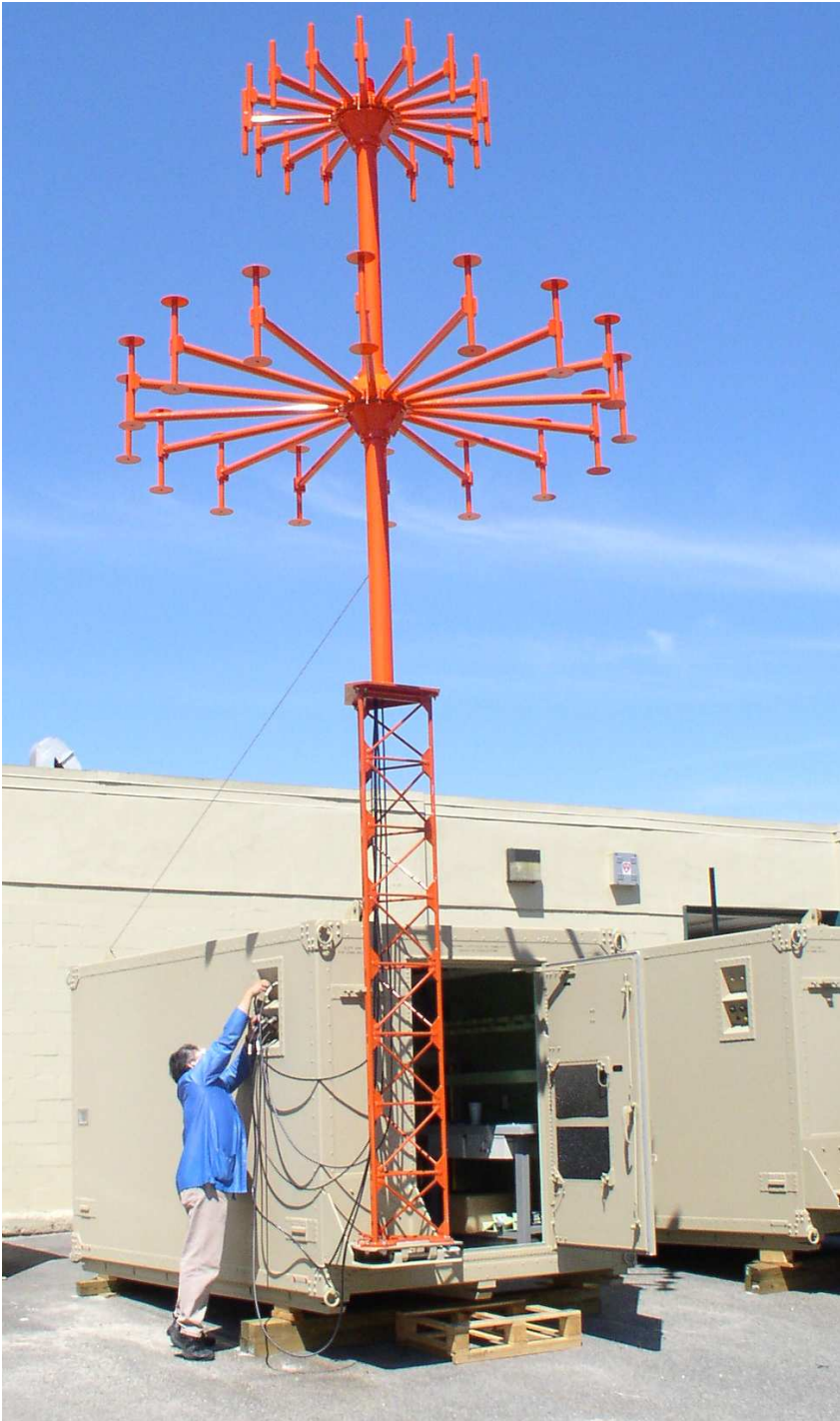
Figure 1-7 DF Antenna mounted on a mobile shelter
