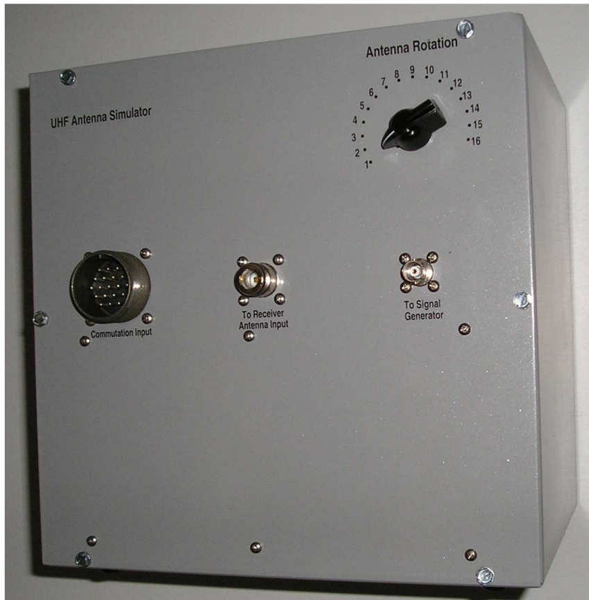
Fig.1 DF UHF antenna simulator
